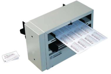
10up business card slitter, easily converts 8 1/2" x 11" sheets to finished 2" x 3 1/2" business cards with a simple two pass operation. Premium features include perfect cuts, catch tray, receptacle and adjustable feed to accommodate different types of material thickness. This unit does not accommodate bleed printing.
