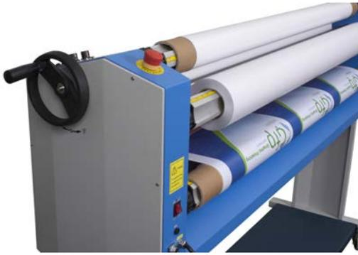
Integrated Rear Rewind makes Roll-to-Roll applications easy.
