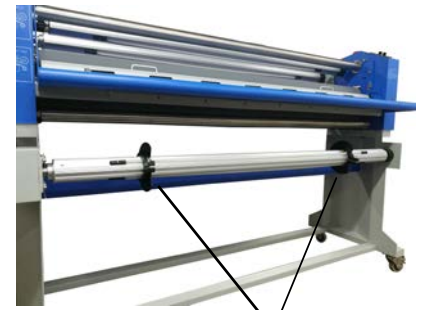
Media Alignment disks keep supply rolls from telescoping
