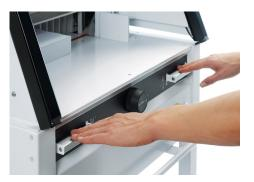
**EASY CUT BLADE ACTIVATION BARS** Patented EASY CUT blade activation bars ensure true, two-handed operation and allow blade and clamp to be activated independently.
